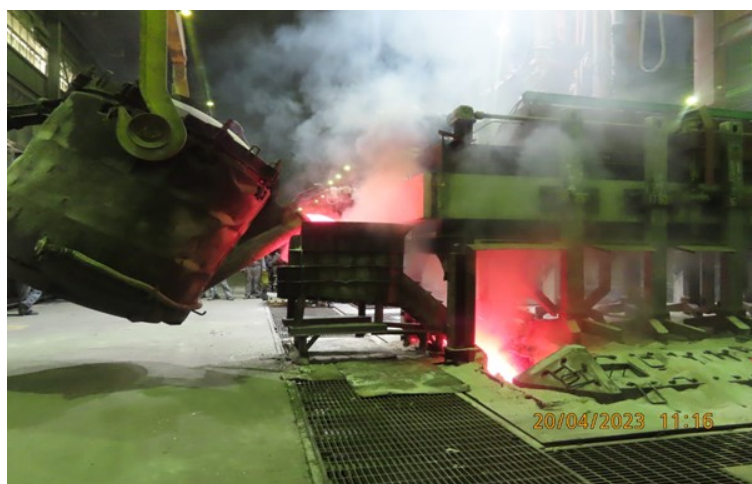
Figure 7. Bath-up in progress.
